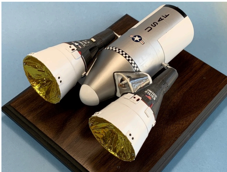
The Military Orbital Development System (MODS) was a proposal in early 1962 for a space station that would use up to two Gemini spacecraft to conduct preliminary research in space. MODS eventually evolved into the Manned Orbiting Laboratory (MOL), which had a dedicated reconnaissance mission and was canceled in summer 1969. (credit: Model and photo by Mike Mackowski)
