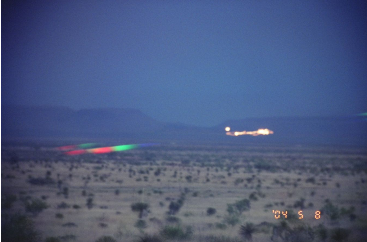
Figure 74 . Photo #17 (ML3c), May 8, 2004, after 9:04pm, Mitchell Flat, Marfa (Texas). Uncropped picture. The rainbow-like pattern is the spectrum of the ML, obtained by using a Mylar diffraction grating insert between the telescopic lens and the camera. © James Bunnell.
