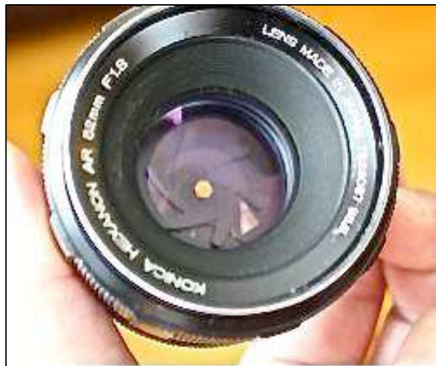
Fig. 257. Six-bladed diaphragm of the Konica AR 52mm lens with hexagonal lens opening. Image borrowed from http://digichar.com/unt/57619-konica_hexanon_ar_52mm_f1_8_lens.html
