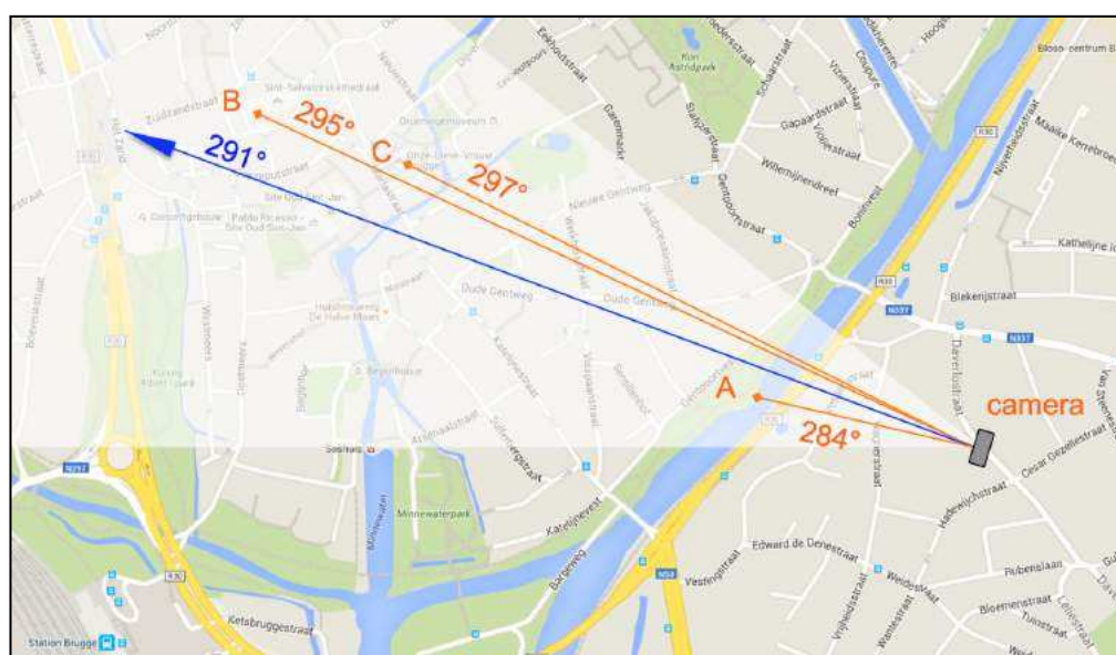
Fig. 225. Map showing the camera's viewing angle for photos #1 and #2 and azimuths for towers A, B and C. The blue arrow designates the azimuth of the unidentified light.
