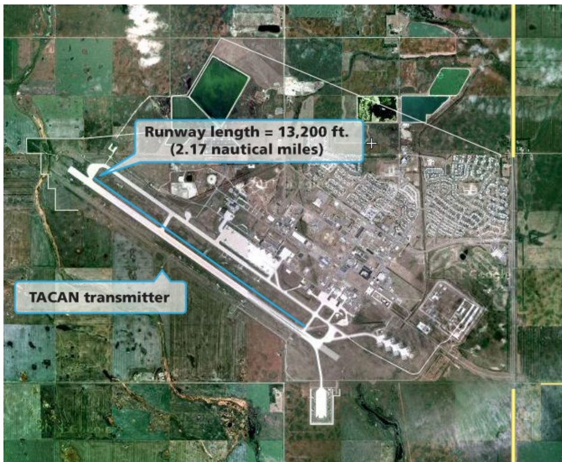
Aerial view of Minot AFB, including the location of the Tactical Air Navigation (TACAN) UHF transmitter beacon. TACAN is an air navigation system that provides an aircrew with the distance (slant-range) of the aircraft, and direction of flight (degrees-of-bearing) to the geographic location of the surface beacon.
