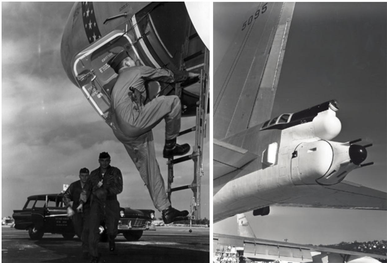
The manned tail gun position of a Wichita-built B-52E with its four, radar-directed .50-caliber machine guns. In this early variant the gunner was isolated in a pressurized cabin in the tail. The B-52H made its first flight on 6 March 1961 and remains in service today. In all, Boeing produced 744 B-52s between 1952 and 1962. ( Boeing ).
